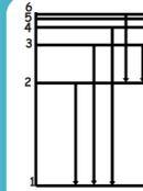
Total no. of different wavelength photons in emission spectrum =  $\frac{n(n-1)}{2}$
